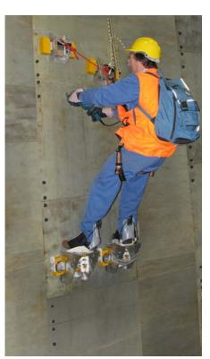
climbed. Electro permanent magnets are used for this purpose. These magnets can be switched between the ON and the OFF state by a short electrical pulse. After the pulse, the magnet remains in the new state without the need of any additional energy. This makes the system inherently safe. The magnets at the feet are operated by a knob in the hand units. For more pictures and a movie, please check www.kleefklimmen.eu
