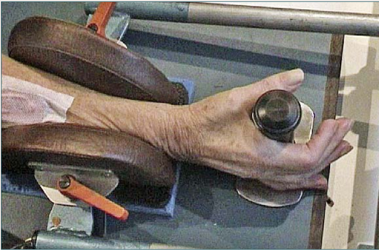
The LUMC in Leiden houses the POPE machine, a device used to measure the performance of PD patients to control their wrist motion. POPE is a derivative of the test setups at TU Delft, and uses an electrical instead of a hydraulic actuator.
