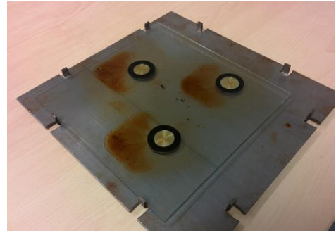
Fig. 1. The figure presents a ferrofluid bearing demonstrator. Three ring magnets with ferrofluid are placed on an iron plate with a glass plate on top of it. The setup shows the ease with which a ferrofluid bearing can be built. The configuration is capable of carrying a load of about 1kg with a bearing surface of only 10cm 2 .
