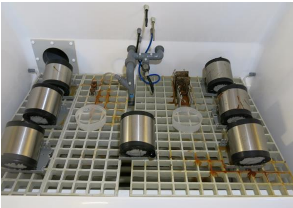
Figure 51: Overview picture of test pieces of laser cladded PTO cylinder in a salt spray test chamber during an accelerated corrosion tests using continuous spraying with natural seawater at a temperature of 28 °C.
