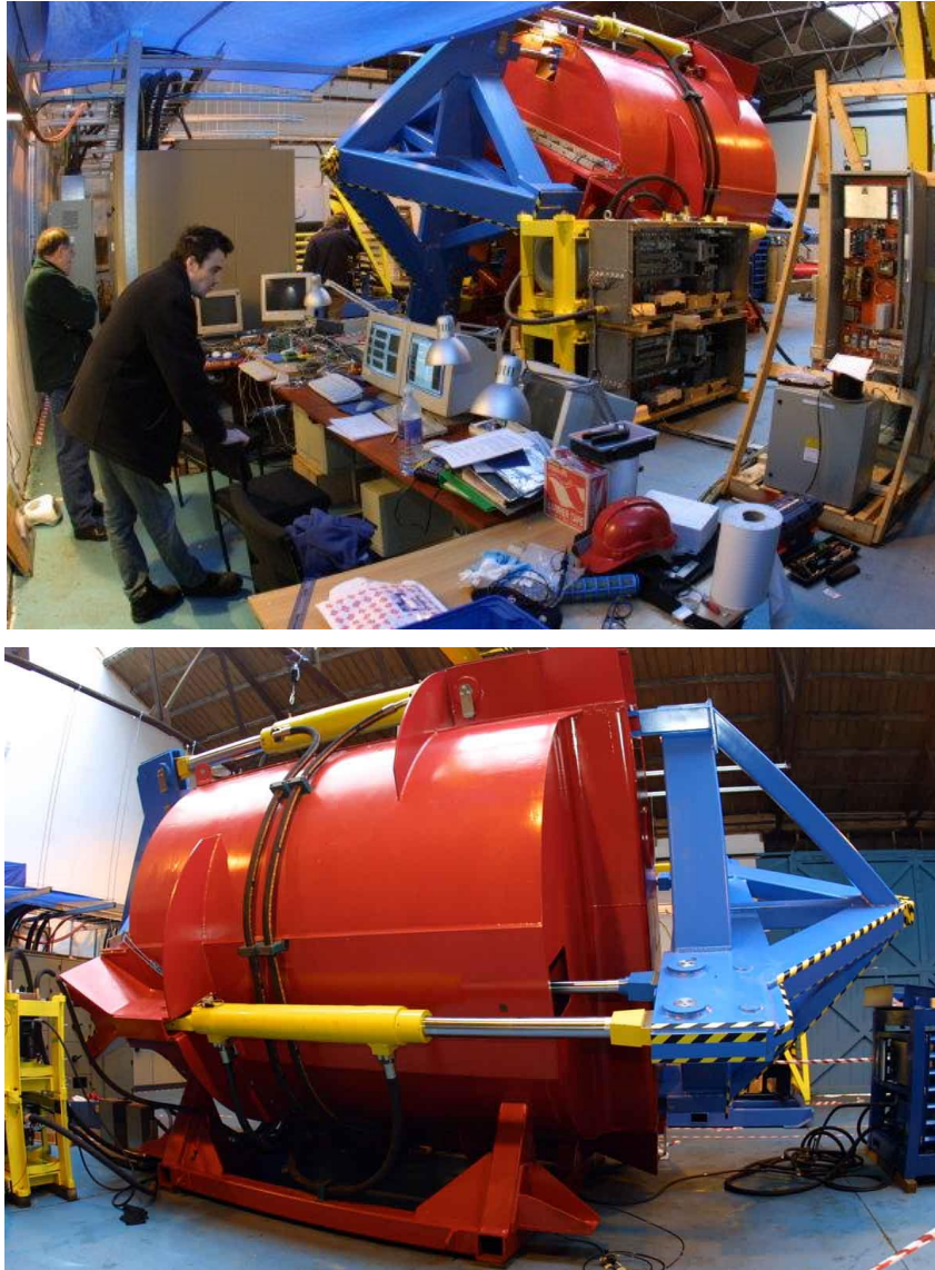
Figure 35: The Pelamis PTO module full-scale test rig [203]
