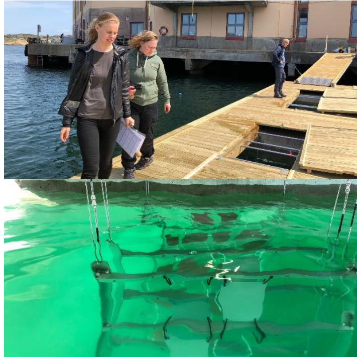
Figure 53: Efficacy evaluation of antifouling products Conduct and reporting of static raft tests for antifouling efficacy (CEPE 2012) @RISE
