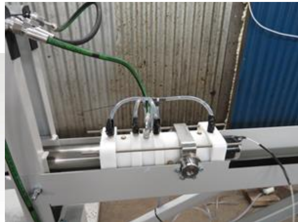
Figure 50: The WavePiston test rig for experimental modelling of wear of dynamic seals.
