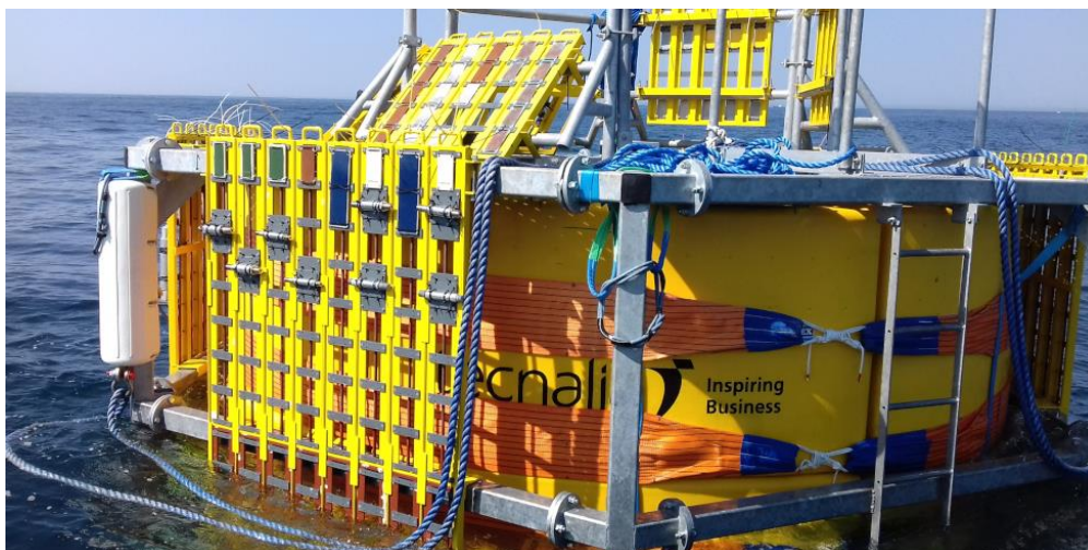
Figure 55: Harslab @TECNALIA. Testing coatings and materials at both immersion zone, splash zone and atmospheric zone.
