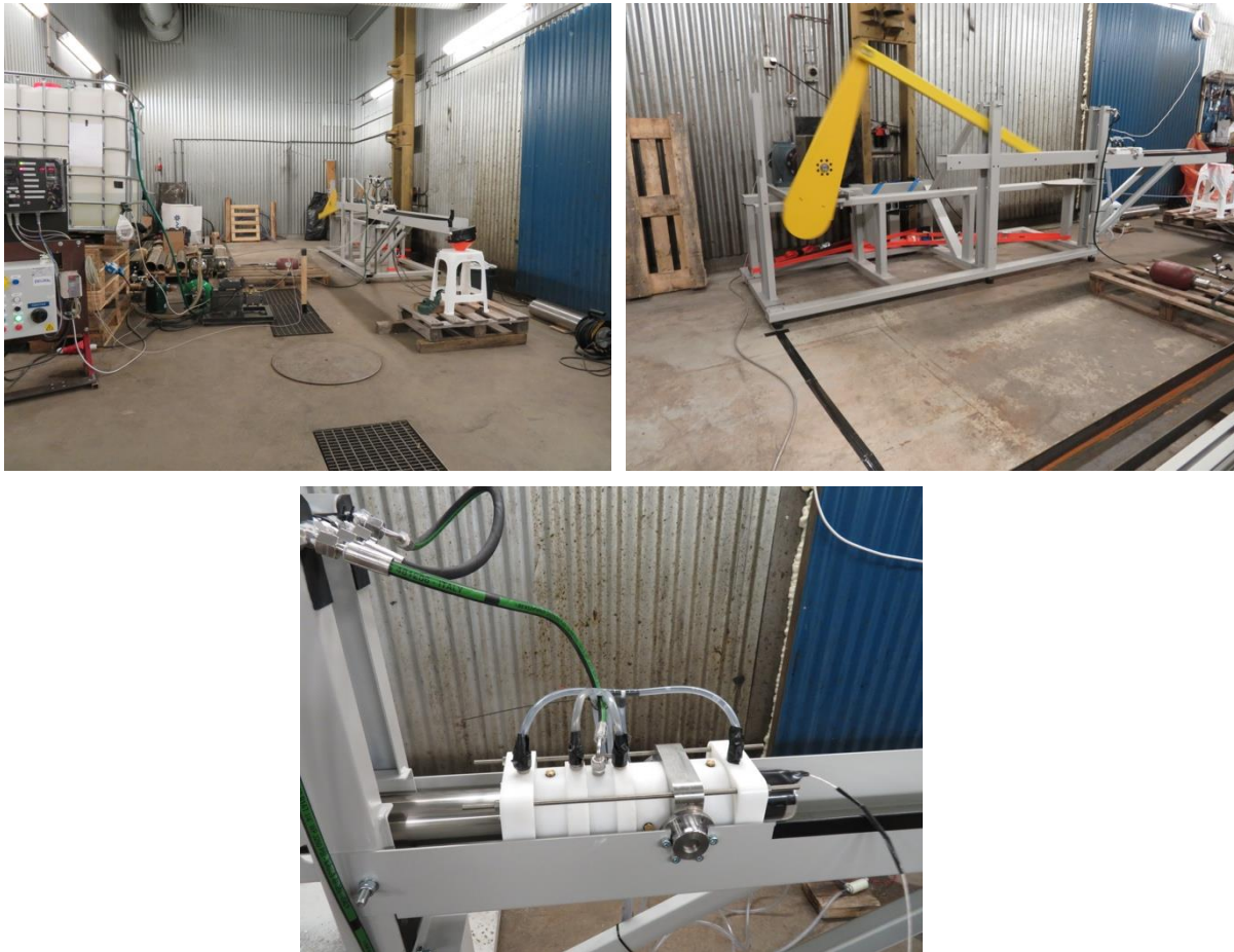
Figure 108: Photos of the Seawater hydraulic pump seal test rig. Top: overview. Bottom: Seal block package.
