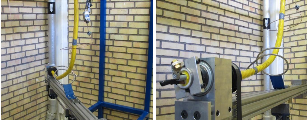
Figure 48: Fatigue testing at RISE in the project “R&D of dynamic low voltage cables between the buoy and floating hub in a marine energy system” [222].
