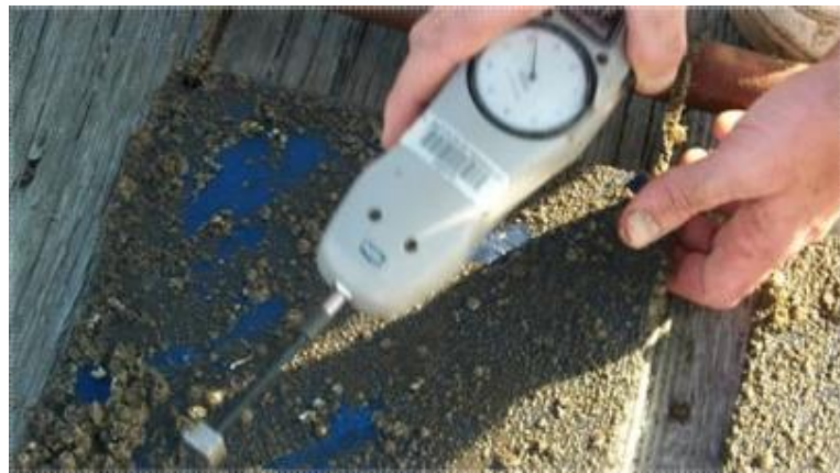
Figure 54: Testing the adhesion strength of barnacles, tube worms and bryozoans on fouling release paints according to the standard method ASTM D5618-20.
