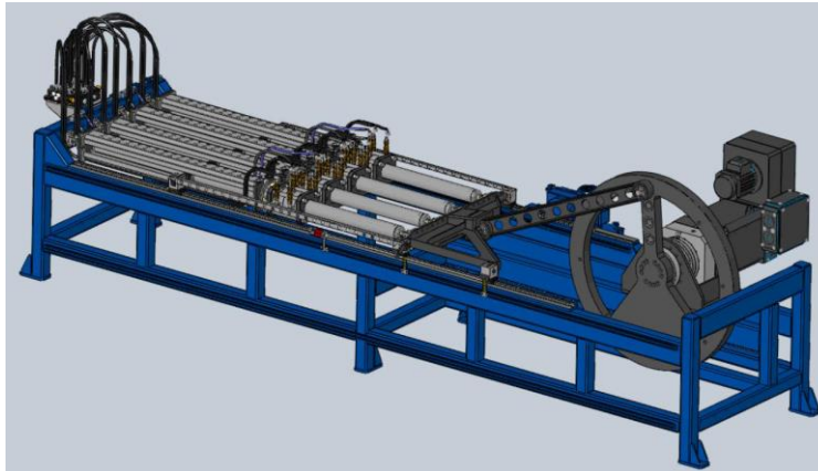
Figure 49: The test rig from the Waveboost project for experimental modelling of wear of dynamic seals [221].
