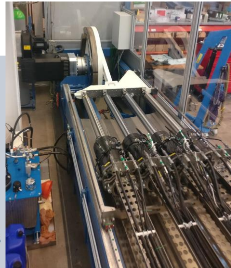
Figure 49: The test rig from the Waveboost project for experimental modelling of wear of dynamic seals [221].
