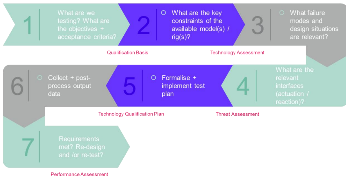
Figure 120: Connection between technology qualification basic steps and key questions associated with a WEC hybrid testing programme
