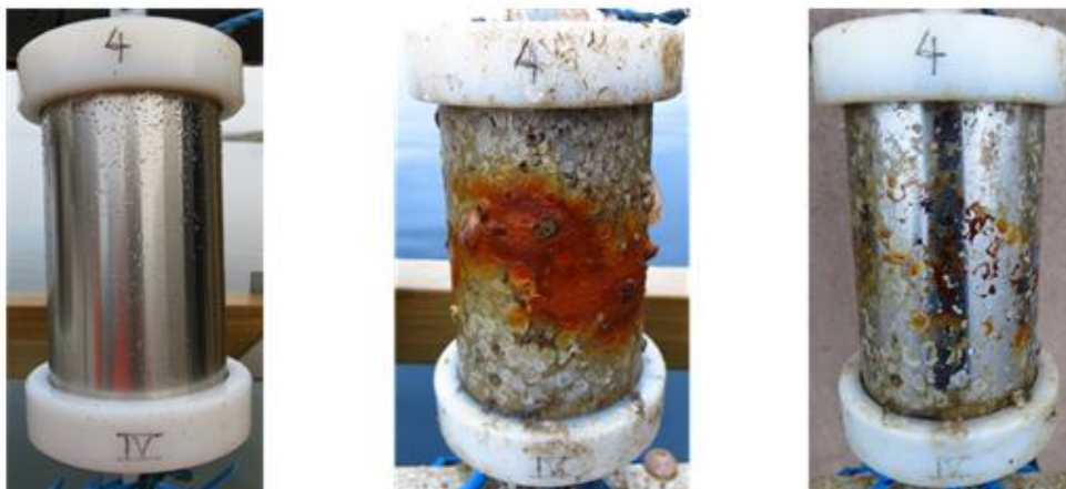
Figure 52: Pictures of a laser clad test piece of a PTO cylinder submerged in seawater under a jetty at Kristineberg test site in Sweden. The stainless-steel coating revealed severe corrosion pits and were of subject to hard biofouling such as barnacles during field test.
